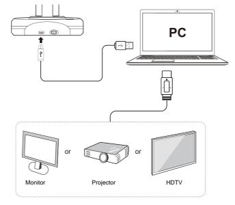
HDMI cable can be connected to monitor, projector, HDTV, and touch screen, etc.
